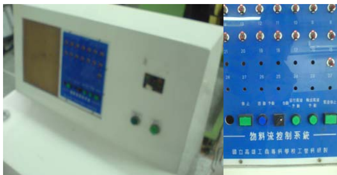
Figure 5. The control desk of the delivery belt
