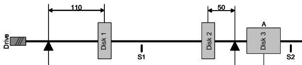
Figure 4. The rotor layout: the displacement sensors at “S1” and “S2” the actuator at “A”. The dimensions are in millimeters.
