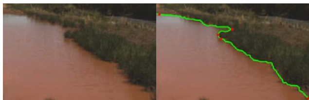
Fig. 7. The GIMP image viewer has an intelligent scissors tool to segment image regions along contours. We have extracted the intelligent scissors portion of GIMP and have integrated it into our ground truthing tool. In this example, only 5 vertices were needed along the cropped portion of the water boundary. Intelligent scissors is run for each pair of neighbor vertices to segment the water's edge.
