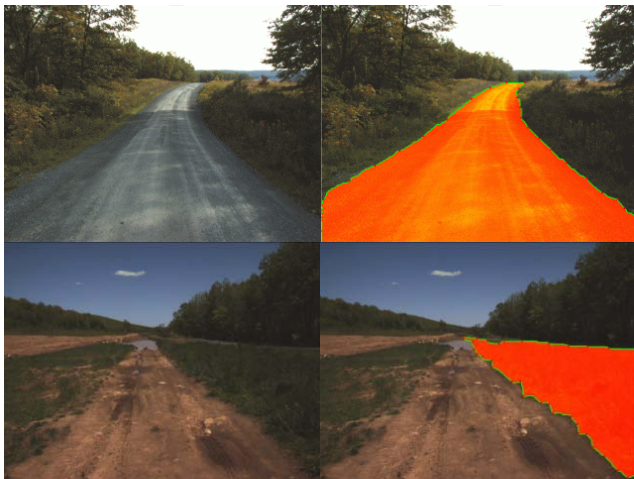
Fig. 19. Examples of ground truthing ground surface terrain types in single frames. In the top row, a gravel road is ground truthed. In the bottom row, a section of short grass is ground truthed.
