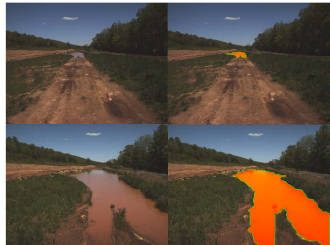
Fig. 8. The water perimeter (green) and labeled water region (orange) for the first and last frame of a 143 frame sequence. This sequence was ground truthed using our software tool. The labeling is quite good, but it is not perfect. For example, it does not exclude interior objects extending out of the water.
