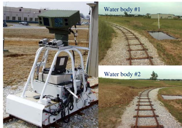
Fig. 14. A JPL passive perception system was mounted to a GDRS instrumented train. Color stereo imagery was collected on a surveyed obstacle course containing two rectangular man-made water bodies at speeds of 1 and 3 m/s.
