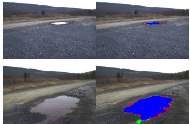
Fig. 11. Water detection results for the first and last image in a 67 frame sequence approaching a shallow water body under an overcast sky. The blue, red, and green pixels indicate true positive detection, false negative detection, and false positive detection, respectively. Water was detected in the first 50 frames by the sky reflection based water detector and the last 45 frames by the color variation based water detector.
