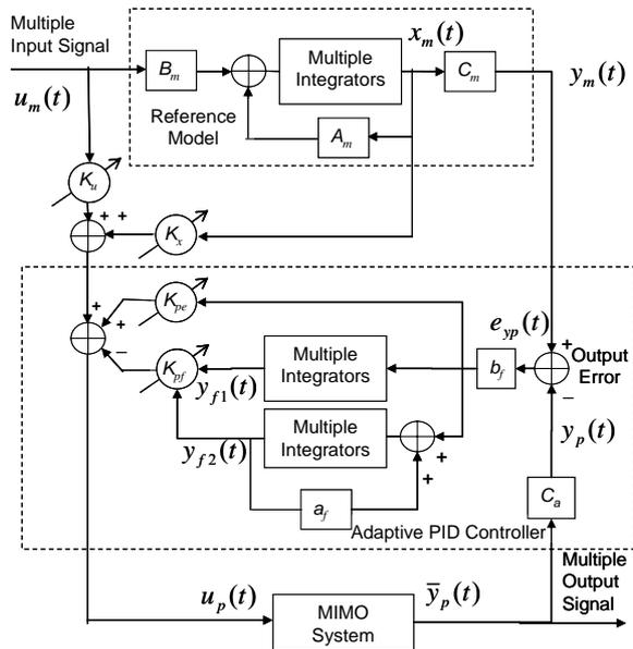
Fig. 2. Output tracking with an adaptive PID controller
