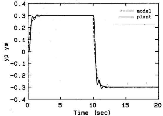
Fig. 6. Output tracking with Adaptive PID Controller
