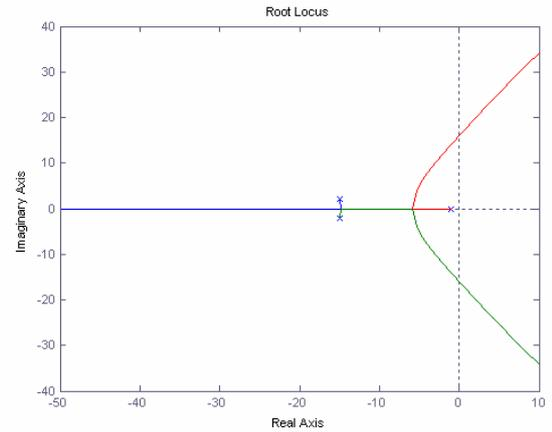
Fig. 3 Root locus plot of Rohrs example
