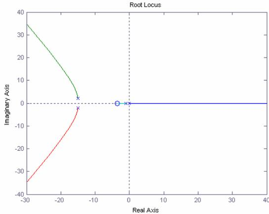
Fig. 4. Root locus plot of Rohrs example with PID
