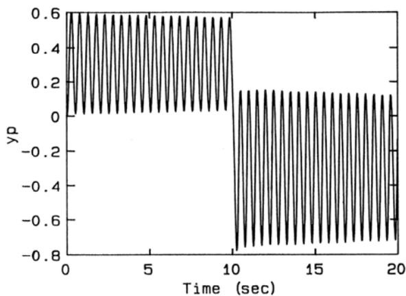
Fig. 5.. Output Tracking with PID Controller
