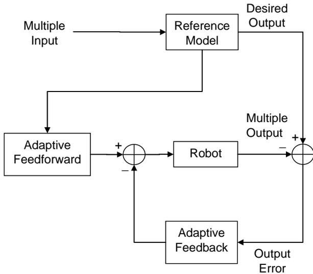
Fig. 1. Robot motion control with a reference model
